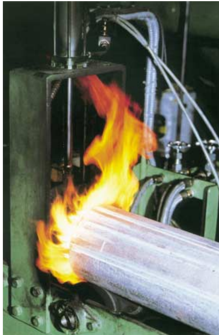
In aluminium bar extrusion the surface is coated with carbon by means of an oxy-acetylene or air-acetylene flame providing a separating and insulating layer. ▶
