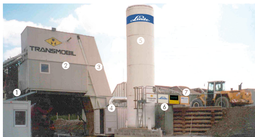
Ready-mixed concrete factory with cooling system during the construction of the Melk railway junction
